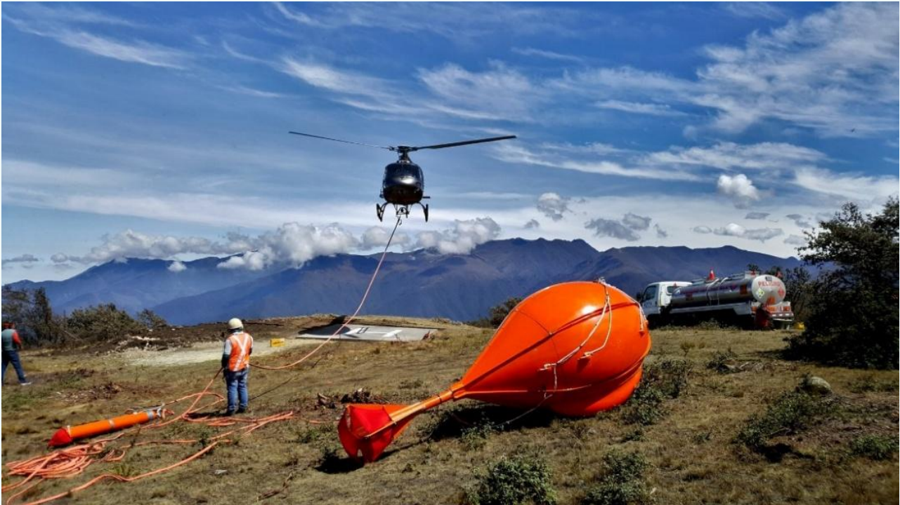
Figure 9. Example of a helicopter with a probe slung for airborne magnetics ( https://expertgeophysics.com/services/ )
