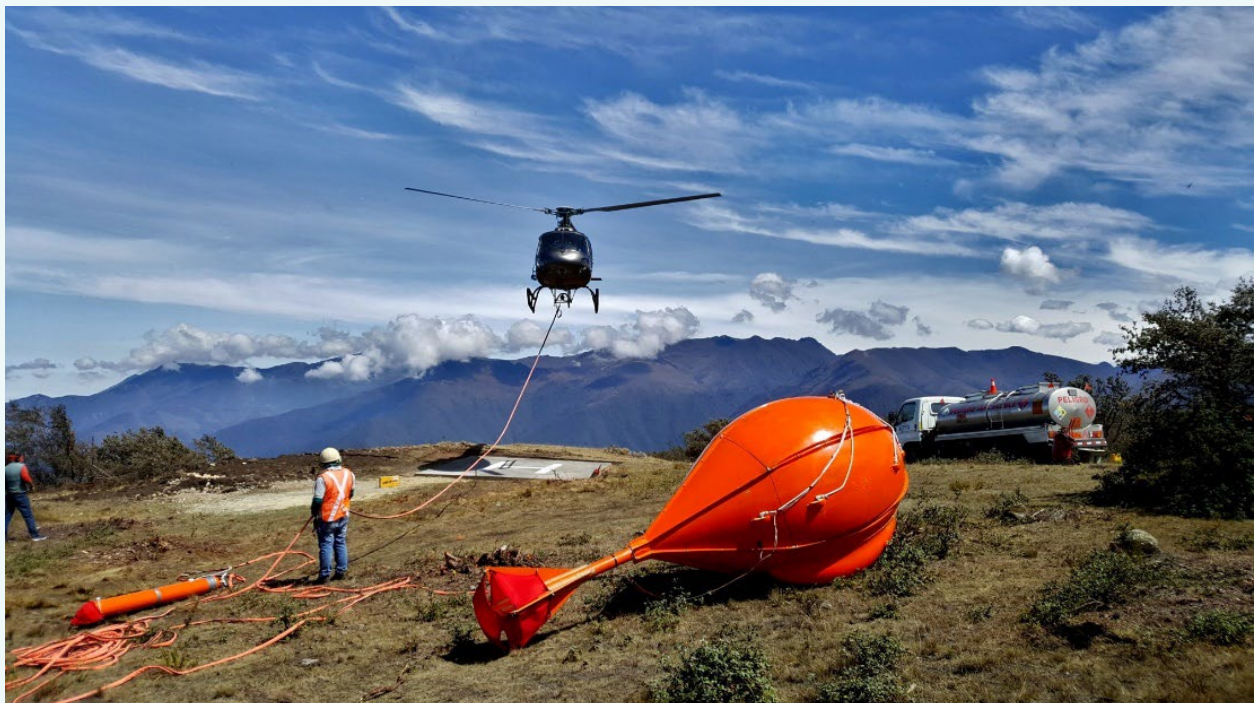
Figure 3. Example of a helicopter with a probe slung for airborne magnetics ( https://expertgeophysics.com/services/ )
