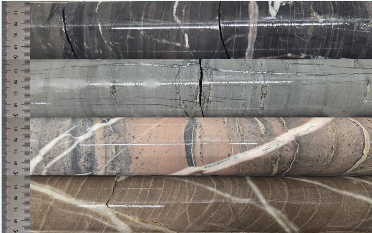
Figure 11. Mineralised horizon in Hole 26-03. From top to bottom: Hanging wall sediments, wispy pyrite-chalcopyrite in altered sediments near contact to below sandstones, pinky coloured alteration zone in sandstones with disseminated to spotty chalcocite-bornite, unmineralised footwall sandstones.
