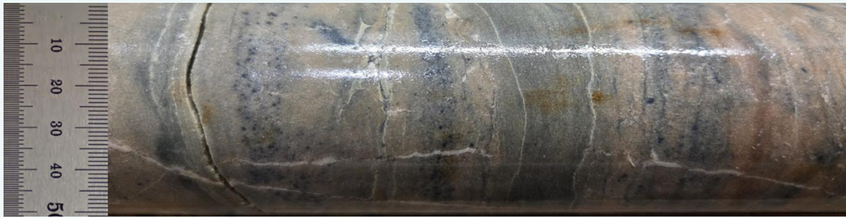
Figure 5. Chalcocite-bornite mineralisation (dark-blue spots in bands) at 225m in Hole 26-02.
