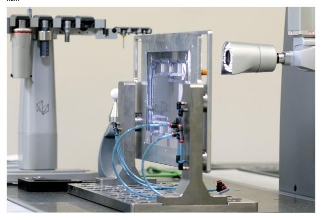
To secure the best possible conditions, the measuring facility is built as a separate entity within the factory in Karlskoga. The slightest vibrations affect the measurement result - as do changes in temperature. Therefore, there is no contact between the room and external walls and the temperature is kept at 20 degrees around the clock, with a permissible variation of 0.4 degrees.
