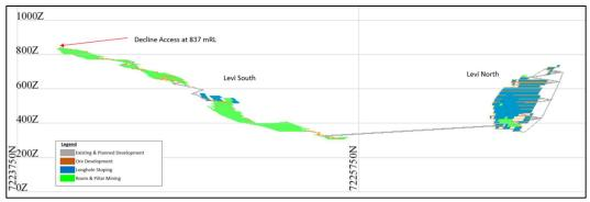
Figure 17: Long view of the Levi Mining Inventory by mining method and existing and planned development, looking southwest
