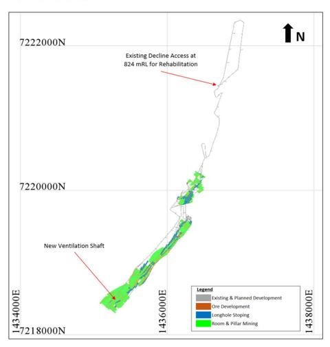
Figure 14: Plan view of the Stekenjokk Mining Inventory by mining method and existing and planned development
