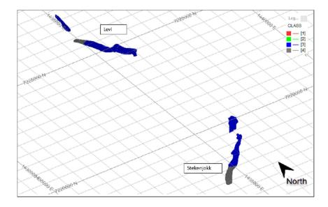
Figure 13: View of the Resource block model for the Stekenjokk-Levi deposit coloured by Classification, blue = Inferred material
