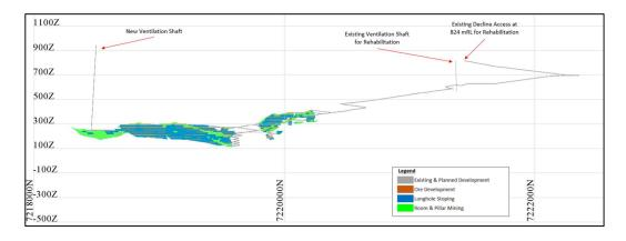
Figure 15: Long view of the Stekenjokk Mining Inventory by mining method and existing and planned development, looking northwest
