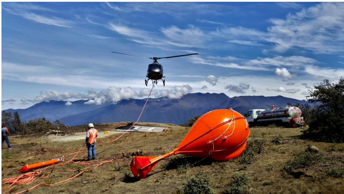
Figure 8. Example of a helicopter with a probe slung for airborne magnetics ( https://expertgeophysics.com/services/ )
