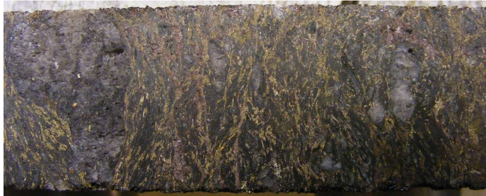
87.1m depth - Sheared and brecciated biotite schist with quartz fragments, rich in sphalerite, galena, chalcopyrite and pyrite stringers (Zn =7.2%)
