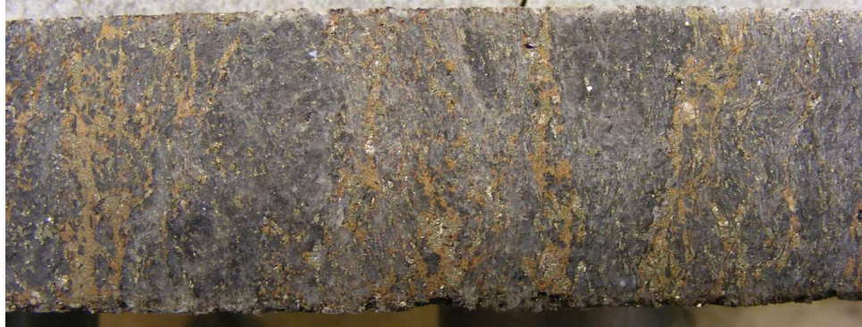
88.05m depth - Quartz rich muscovite biotite gneiss, rich in dissemination stringers of sphalerite, galena, chalcopyrite and pyrite (Zn =5.5%)
