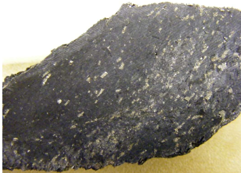
20.45m depth – 8 cm wide biotite shear with pyrite, chalcopyrite, galena, sphalerite dissemination and minor Au.
